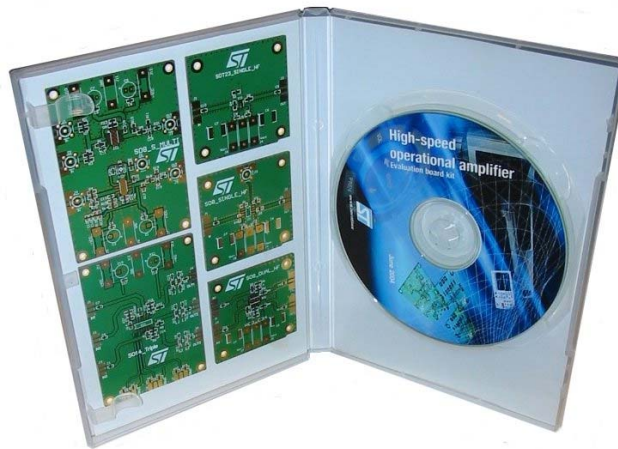
Figure 44. Evaluation kit for high-speed op-amps
